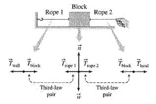
What does Newton's third law say about the tension forces exerted by the block on the two ropes?
