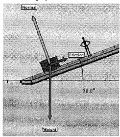
Watch what happens to the force of friction (the red vector in the picture or the red plot in the graph) before the crate starts to slide down the ramp.
