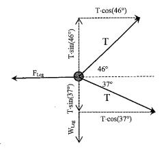
The only unknowns in the two equations above are T and  $F_{\text{Leg.}}$  So a solution is possible for the two simultaneous equations. Substitute W for T and 51.5 N for  $W_{\text{Leg.}}$  Solve for W and  $F_{\text{Leg.}}$
